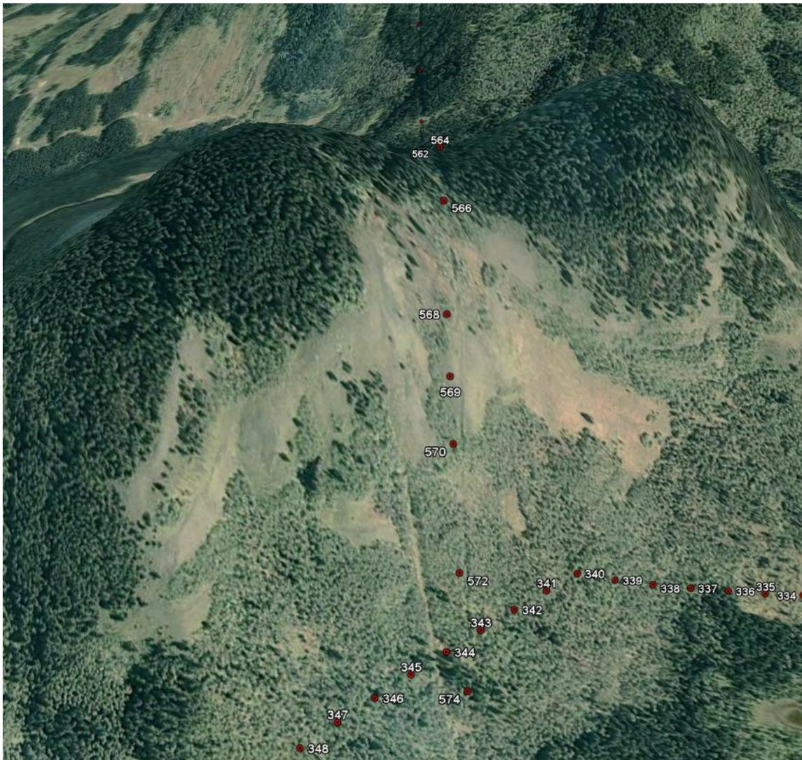
As shown below (rotated view, looking west), any movement to fit the cutline, clearly visible at the bottom, will dramatically impact the location of station 564 on top of the mountain.
